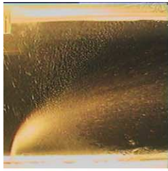
(a) Photographic image of the Venturi throat with a single jet for u_g = 58.3 m/s and u_j = 6.07 m/s.
